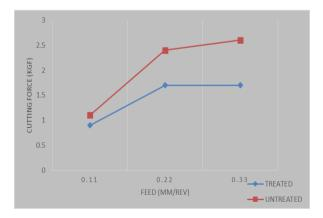
It was found that the cutting force of the treated tool decreased by an amount of 35% in comparison with the untreated tool.
