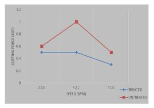
It was found that the cutting force of the treated tool decreased by an amount of 44% in comparison with the untreated tool.
