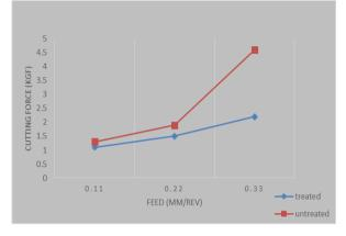
It was found that the cutting force of the treated tool decreased by an amount of 30% in comparison with the untreated tool.
