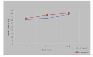
It was found that the tool tip temperature decreased by an amount of 8% in comparison with the untreated tool.
