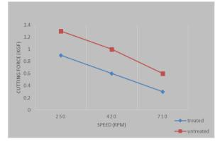
It was found that the cutting force of the treated tool decreased by an amount of 40% in comparison with the untreated tool.
