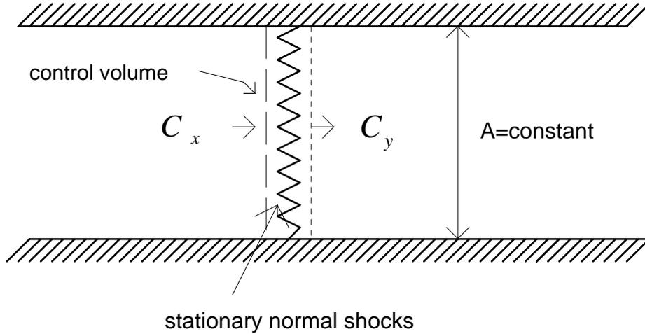
Figure shows a normal shock wave in a constant area frictionless duct, the shock wave is considered to be contained in a control volume.
