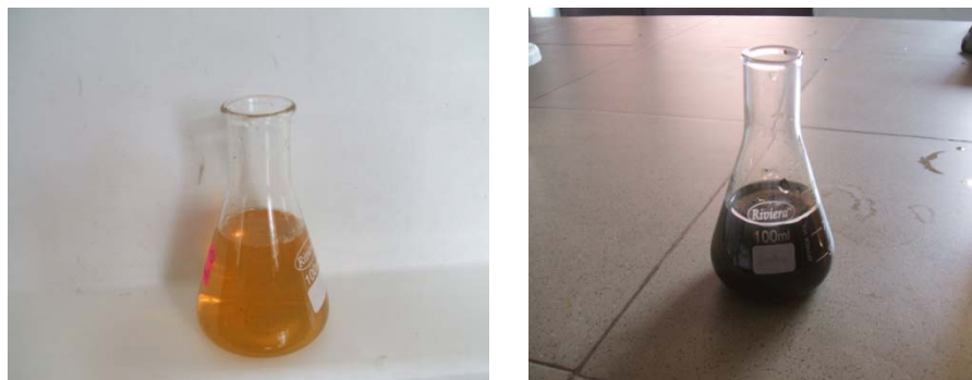
Figure 1: (A) Epicarp extract, (B) Colour changed after 24 hours incubation of extract with 10^{-3} M solution of \text{AuCl}_4 .
