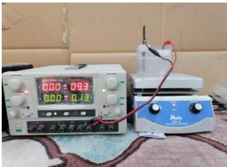
Figure 1: The Al 2 O 3 /ZnO Nano composite is prepared using an electrochemical method.
