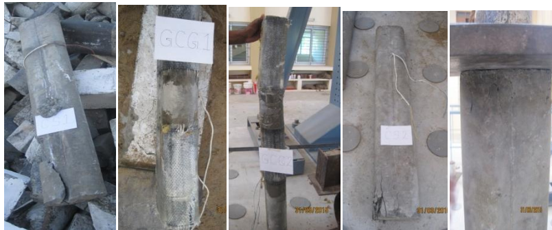
Fig 7 Failure Pattern of tested Specimens
