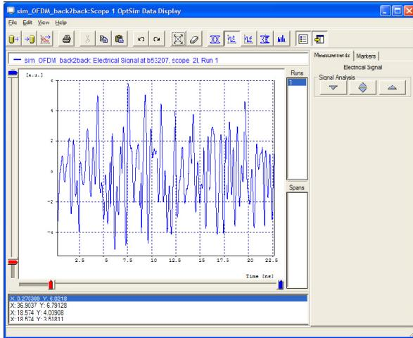
**Figure 5:** In-phase component of OFDM signal at scope\_2I.
