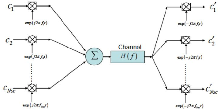
**Figure 1:** Conceptual diagram for a generic multi-carrier modulation (MCM) system.
