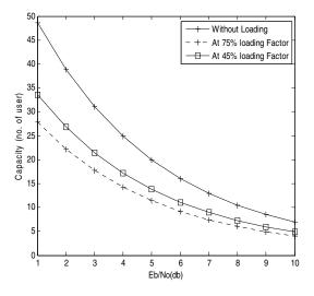
Figure 2: Effect of Loading on WCDMA capacity for video services.
