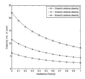
**Figure 9:** Effect of antenna Diversity on WCDMA capacity with  $\beta$ =0.4 & 100% loading for 768kbps data rate applications.
