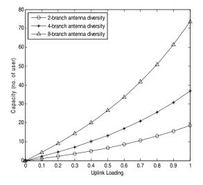
**Figure 6:** Effect of antenna Diversity on WCDMA capacity with  $\beta$ =0.7 & i=0.6 for 144kbps data rate applications.
