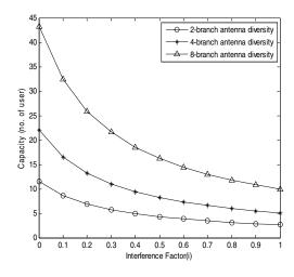
**Figure 8:** Effect of antenna Diversity on WCDMA capacity with  $\beta$ =0.7 & 100% loading for 768kbps data rate applications.
