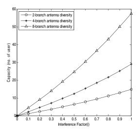
**Figure 7:** Effect of antenna Diversity on WCDMA capacity with  $\beta$ =0.4 & i=0.6 for 144kbps data rate applications.
