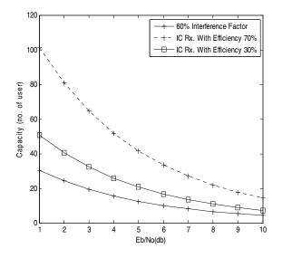
**Figure 5:** Effect of Interference Cancellation (IC) Receiver on WCDMA capacity for video application.
