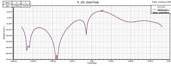
Figure 7.1: 2D gain of antenna for LCP-Substrate.
