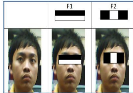
Fig. 4: Chain of single haar-like feature filter in frontal face detection.
