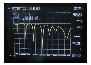
Figure 6: Measurement of Return Loss At4.3ghz
