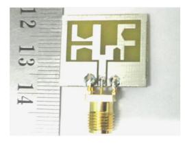
Figure 2: Fabricated bevel U-L shaped antenna
