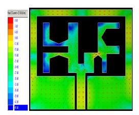
Figure 6(a): Surface Current Distribution at 4.3GHz
