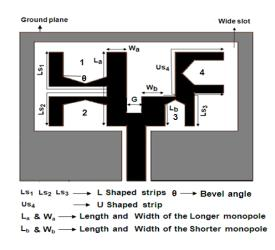
Figure 3: Parameters of bevel U-L shaped antenna
