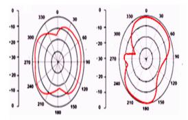
Figure 7 (a): Radiation pattern at 4.3 GHz and 7.4 GHz E-plane (XZ)
