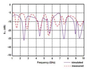
Figure 4: Return loss Characteristics of a bevel U-L shaped antenna
