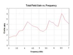
Figure 8: Gain Characteristic of a bevel U-L shaped antenna
