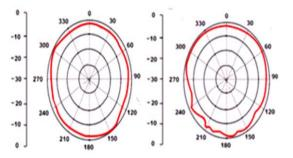
Figure 7 (b): Radiation pattern at 4.3 GHz and 7.4 GHz H-plane (XY)
