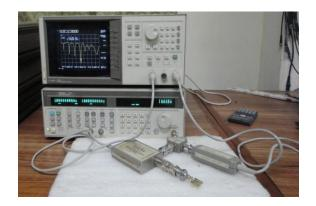
Figure 5: Return loss measurement using HP 8757D Scalar NW Analyzer for a bevel U-L shaped antenna
