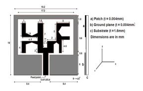
Figure 1: Geometry of The Proposed Antenna
