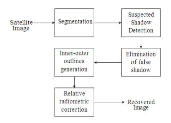
Fig. 1. Block diagram of shadow detection and removal
