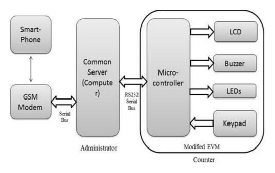
Fig.2: Architectural Block Diagram
