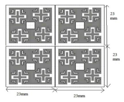
Figure 4: Two dimensional arrays of patches with different slots
