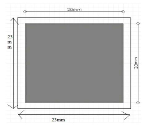
Figure 2: Unit cell of conventional FSS structure
