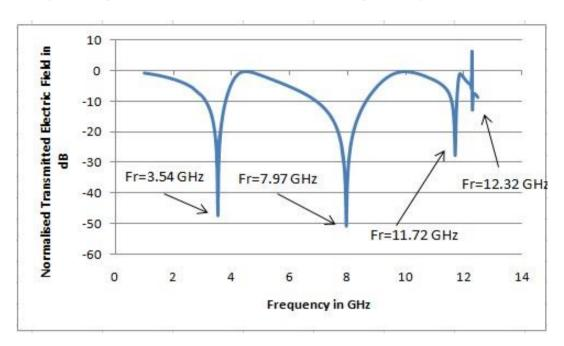
Figure 6: Study of normalized transmitted electric field vs. frequency (corresponding to FSS of Fig.3)
