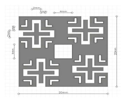
Figure 3: Unit cell of the proposed FSS structure
