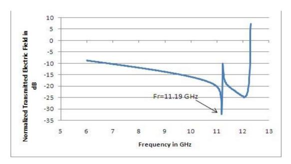
Figure 5: Study of normalized transmitted electric field vs. frequency (corresponding to FSS of Fig.2)
