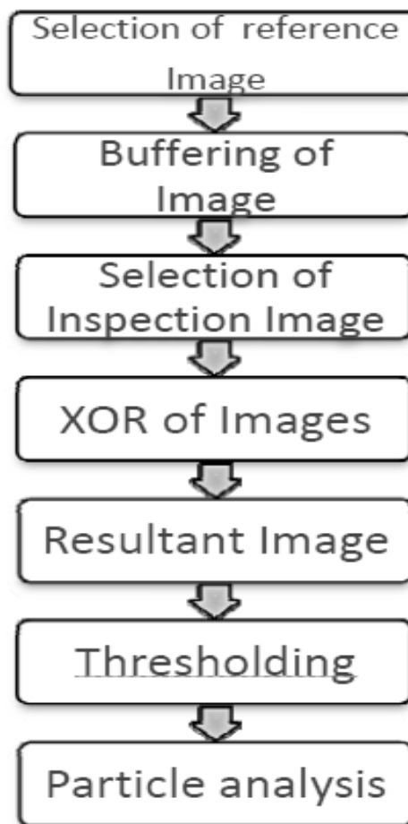
Figure 5: Inspection flow chart-I
