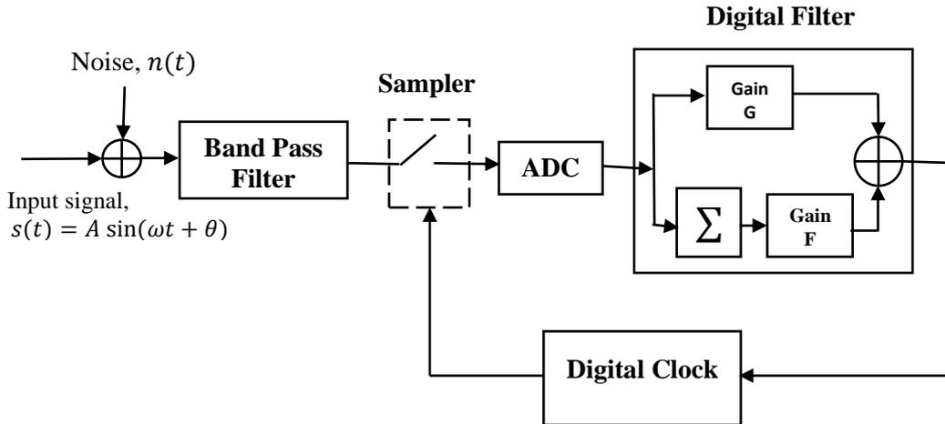
**Fig. 1:** Block diagram of ZCDPLL
