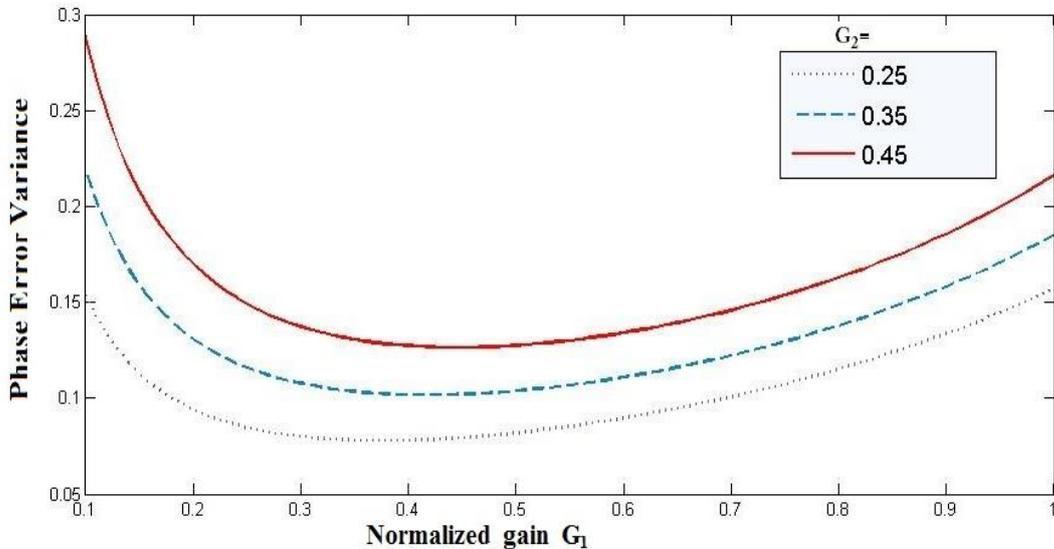
**Fig.3-** Plot of Phase error variance V/s Normalized gain  $G_1$  for different  $G_2$  ;  $R=5$
