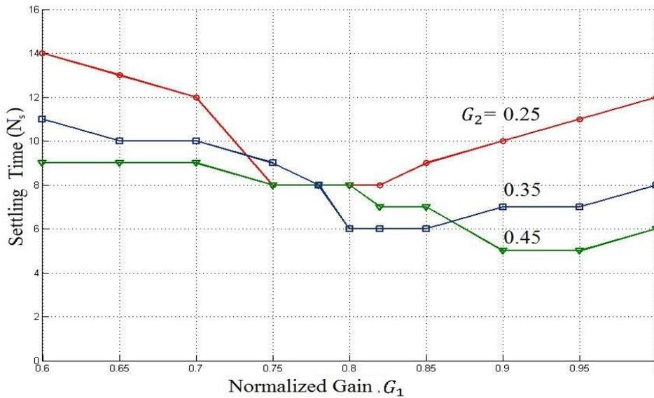
**Fig.2-** Variation of Settling Time with Normalized Gain ( $G_1$ ) for different  $G_2$
