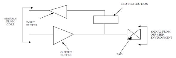
FIG 1: BLOCK DIAGRAM OF BIDIRECTIONAL BUFFER
