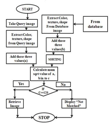
Figure 4: Flow chart of local ternary pattern for content based image retrieval
