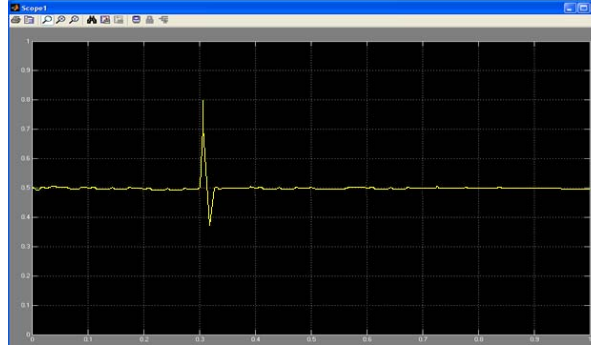
Figure 6(a): Plot of I_{dc} for single line to ground fault with Fuzzy Controller.
