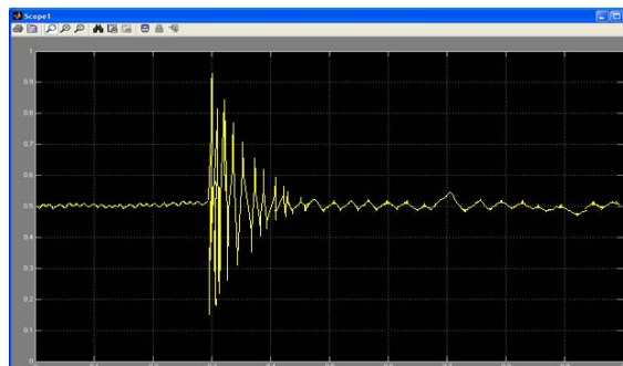
Figure 5 (b): Plot of I_{dc} for single line to ground fault with PI Controller.
