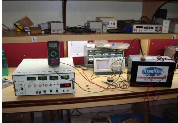
**Figure 9:** Constant current charging of 24PP30 super capacitor.
