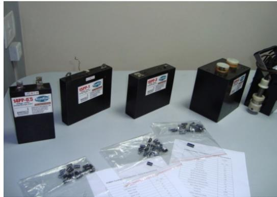
**Figure 4:** Different types of supercapacitors.
