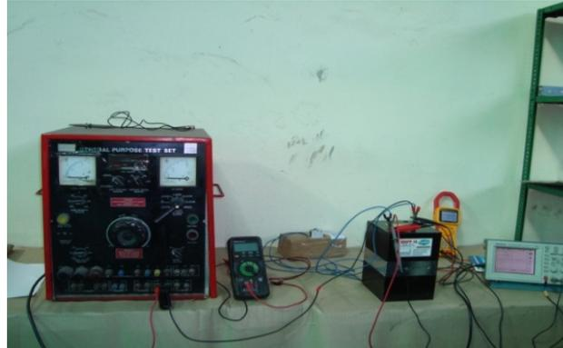
**Figure 5:** Charging and Discharging set up of 100PP14.
