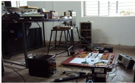
**Figure 17:** Overall hardware circuit of 100PP14 super capacitor with grid connected three phase inverter.
