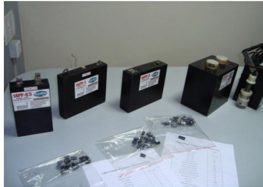
**Figure 4:** Different types of supercapacitors.
