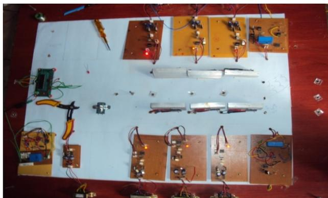
**Figure 15:** Working model of gate drive circuit controlled by PIC16F877A.
