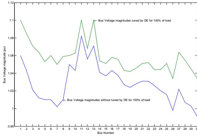
Voltage Profile of the system for Case 1
