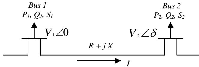
**Figure 1:** Two-bus power system model
