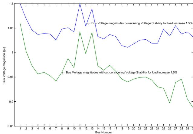
Voltage Profile of the system for Case 3
