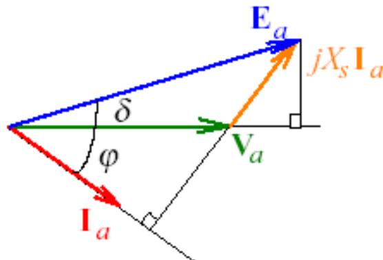
Figure 2: Generator Phase Diagram.
