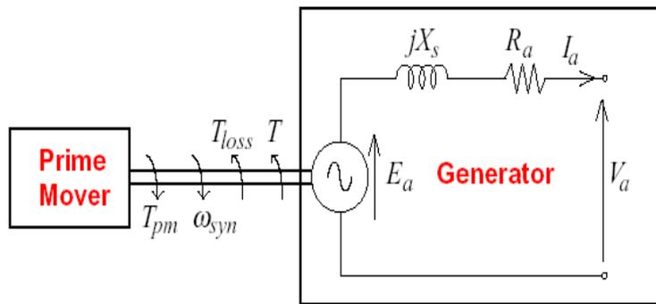
Figure 1: Synchronous Machine operated as generator
