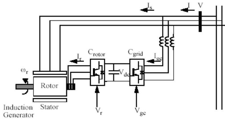
**Figure 3:** Rotor-side and grid side converters.
