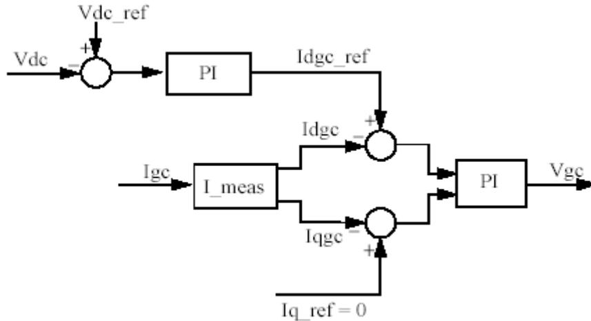
**Figure 5:** Grid-side controller.
