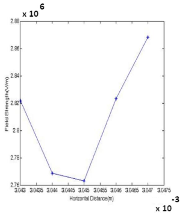
**Figure 9:** Electric Field inside the water bubble for Capacitive graded cable 10kV
