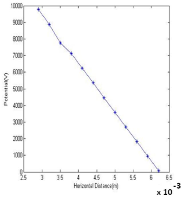
**Figure 11:** Potential distribution on the radial line for Capacitive graded cable 10kV
