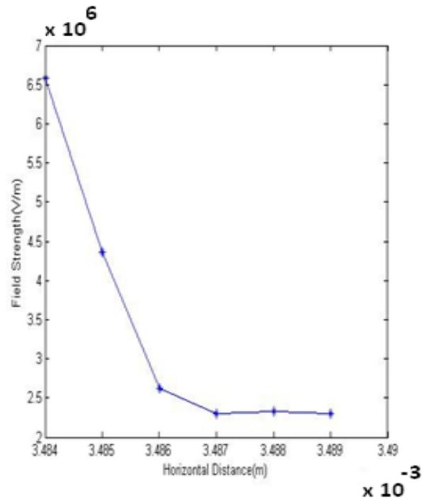
**Figure 8:** Field Strength on the curved surface water bubble for Capacitive graded cable 10kV
