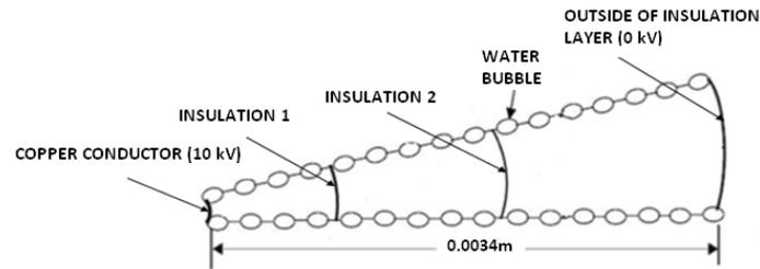
**Figure 3:** Cable section comprising water bubbles in symmetrical configuration\_10kV
