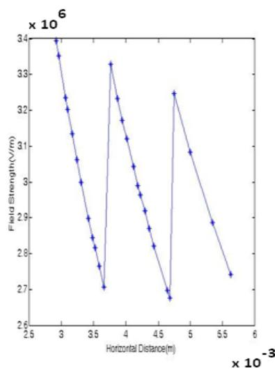
**Figure 5:** Electric field variation in dry capacitive graded cable for 10kV
