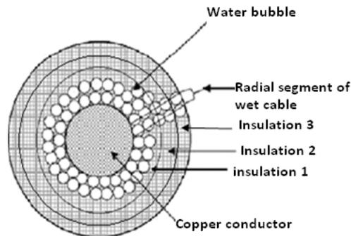
**Figure 2:** Simplified representation of the proposed model of water content in the cable insulation
