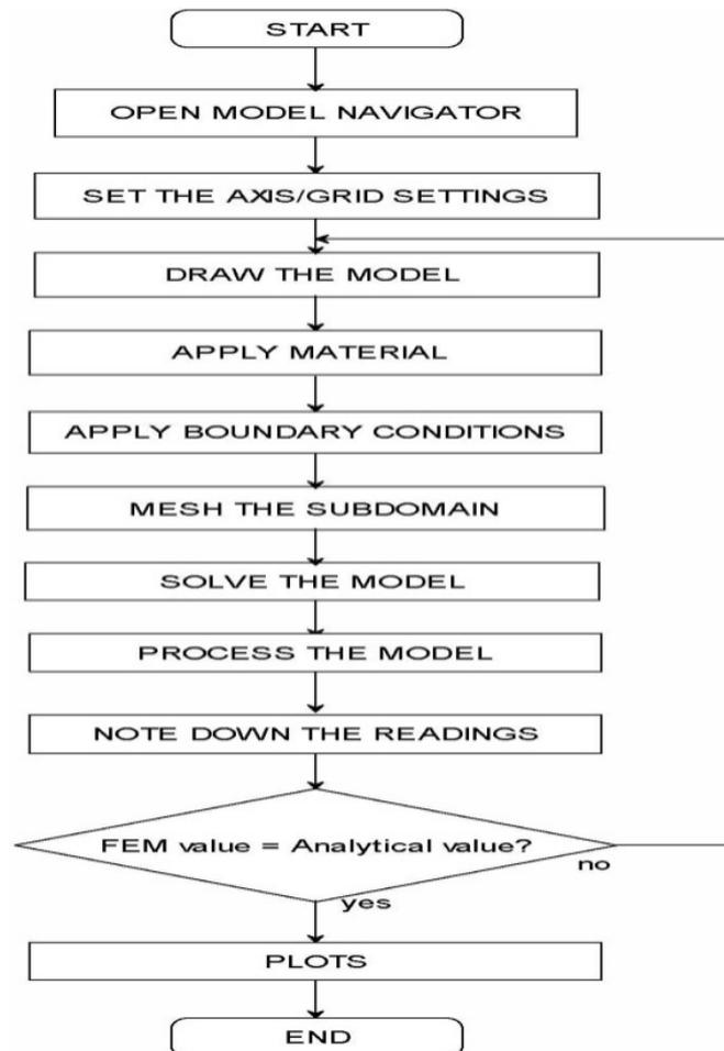
**Figure 12:** Sailing the model through comsol multiphysics
