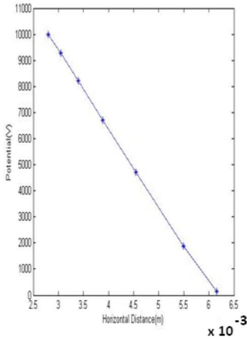
Figure 6: Potential distribution in dry capacitive graded cable for 10kV
