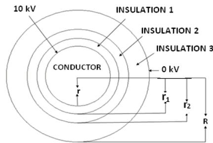
**Figure 4:** 10kV graded co-axial power cable
