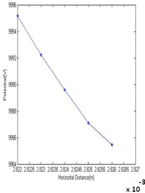
Figure 7: Potential distribution inside the water bubble for Capacitive graded cable 10kV
