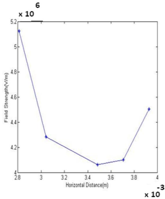
**Figure 10:** Field at the tip of the water bubble for Capacitive graded cable 10kV
