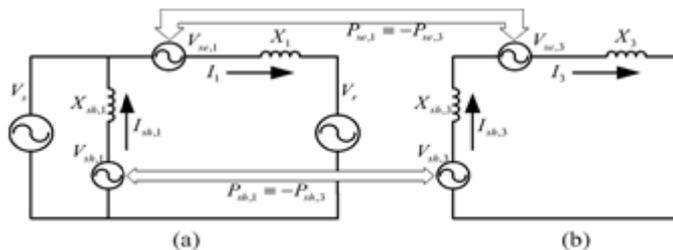
**Figure 9:** DPFC equivalent circuit: (a) the fundamental frequency; (b) the 3rd harmonic Frequency
