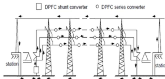
**Figure 3:** 3rd Harmonic Current flow in DPFC
