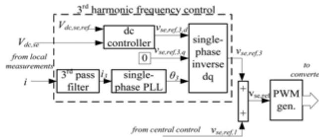
**Figure 6:** Block diagram of the series converter control [8].
