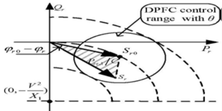
Figure 11: Relationship between  $P_{se,1}$  and the power flow at the receiving end
