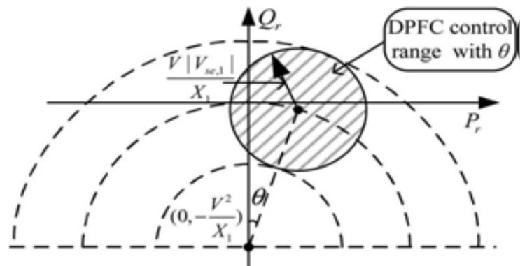
Figure 10: DPFC active and reactive power control range with the transmission angle  $\theta$ .
