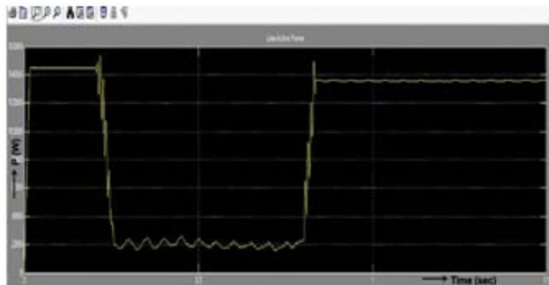
**Figure 20:** Line active power for without DPFC
