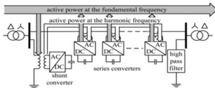
**Figure 2:** Active power exchange between DPFC converters.
