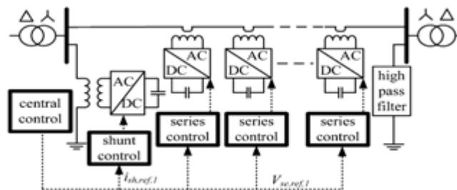
**Figure 5:** DPFC control block diagram.
