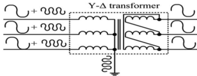
**Figure 4:** Utilize grounded Y- $\Delta$  transformer to filter zero-sequence harmonic.
