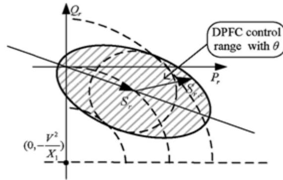
**Figure 13:** DPFC power-flow control range.
