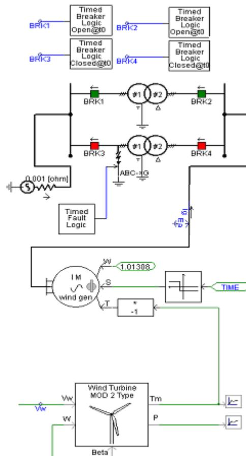
**Figure 5:** Simulation Model for Wind Turbine Generator
