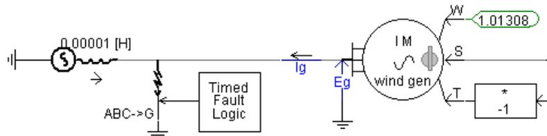
**Figure 4:** Three phase grid fault simulation
