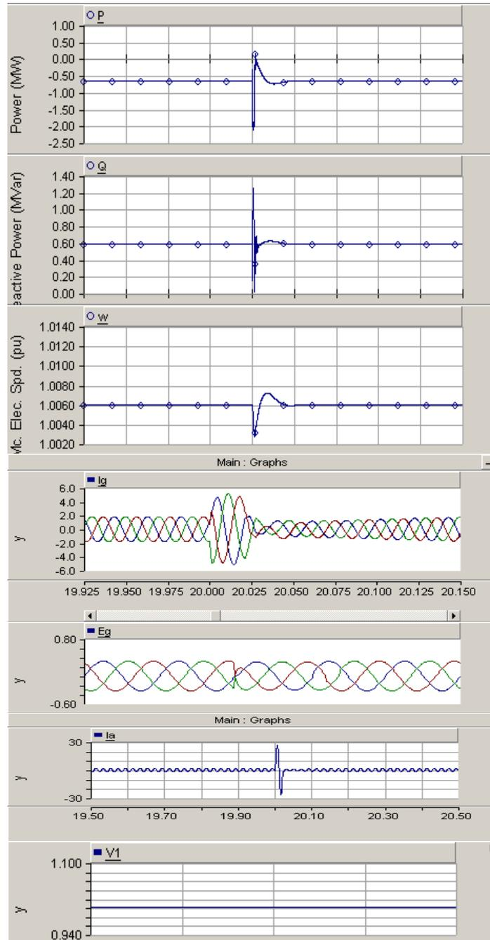
**Figure 6:** Simulation results during the faulty grid
