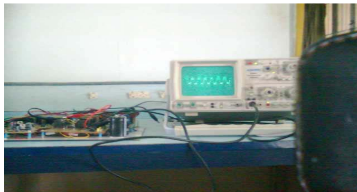
Figure 7: Configuration of four switch BLDC motor drive
