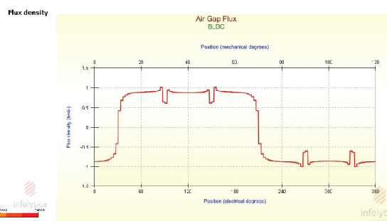
Fig 2 Flux when airgap = 0.3mm
