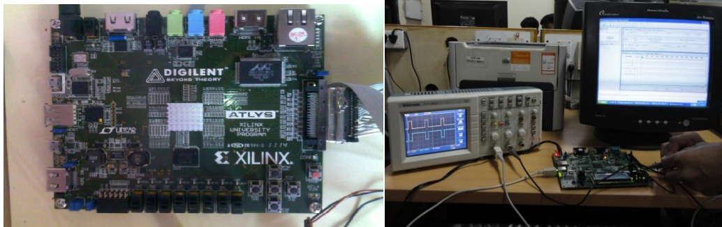
Figure 4 (a), (b): Gate pulses generated using FPGA as digital controller
