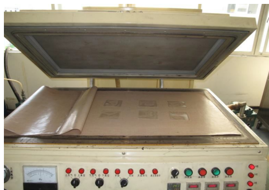
Figure.6 Lamination Machine for PV Cell
