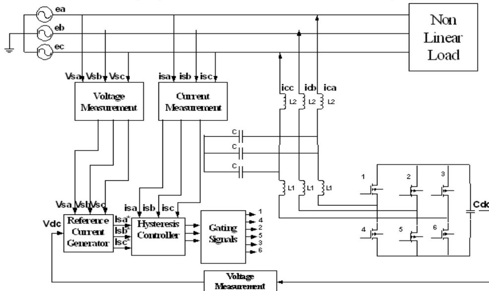
Figure 3: SAPF Block Diagram with Indirect Current Control Technique.
