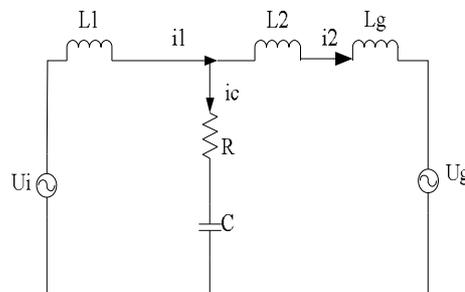
**Figure 2:** LCL Filter Equivalent Circuit.
