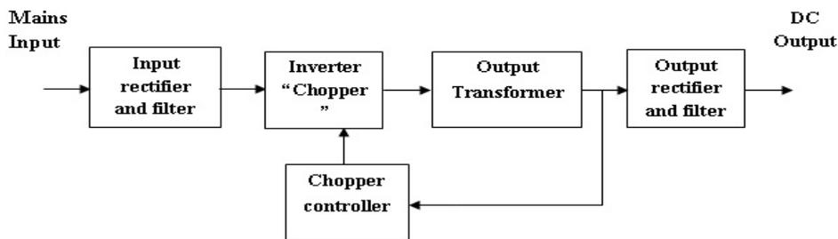
Figure 5: Block Diagram of SMPS.
