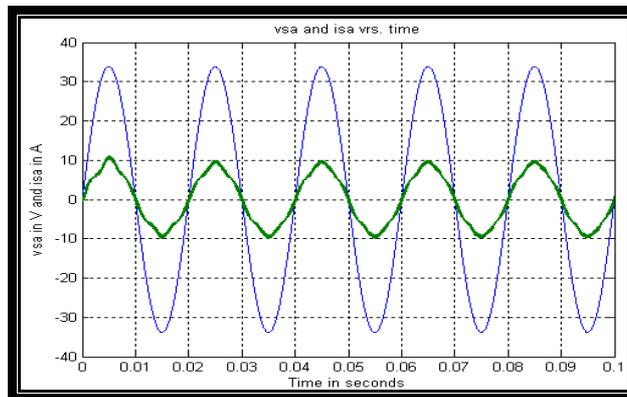
**Fig.15: Grid phase-a voltage and current with  $R-L$  load after operation of the STATCOM**
