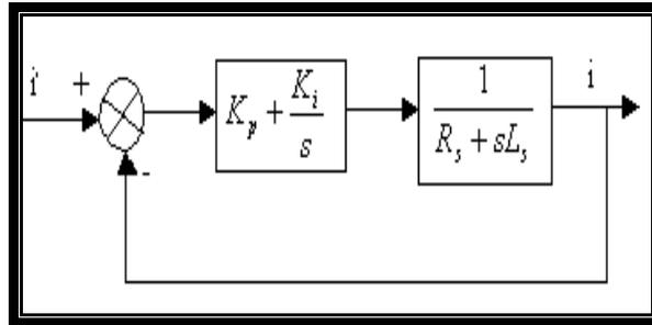
Fig.5: Effective closed loop current control system
