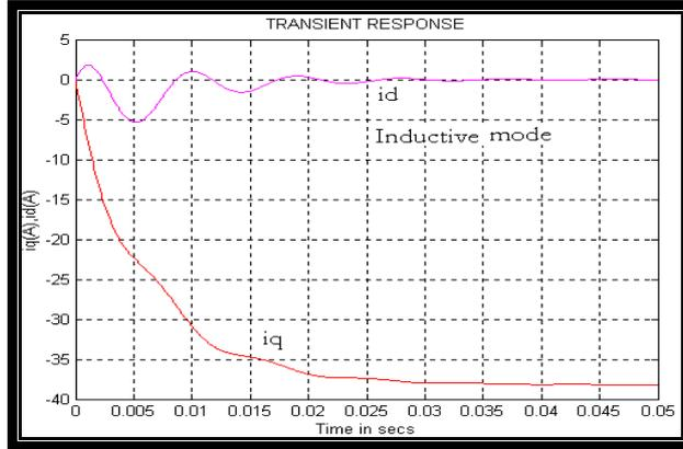
**Fig.9: Transient response of  $i_d$  and  $i_q$  in inductive mode**
