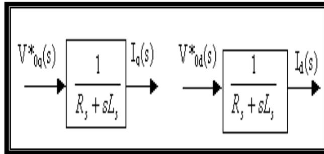
**Fig.3: Current control of inverter of equivalent decoupled SISO systems**
