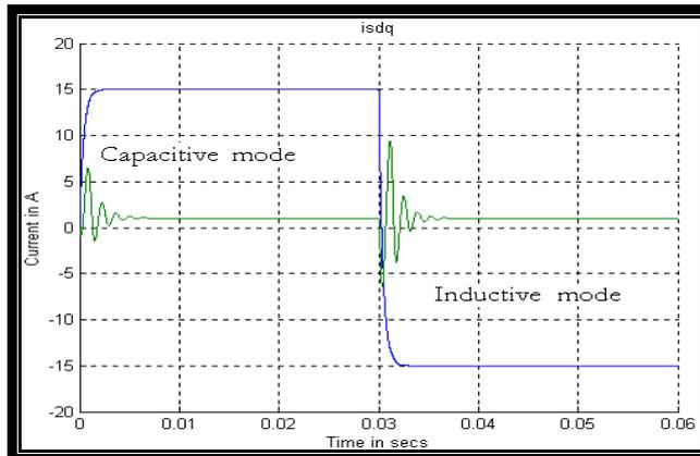
**Fig.11: Current control with reference**
