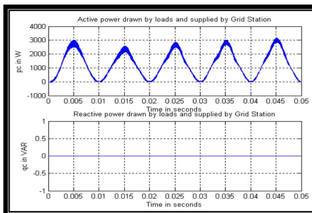
**Fig.16: Grid supplied active and reactive power to  $R-L$  load after operation of the STATCOM**
