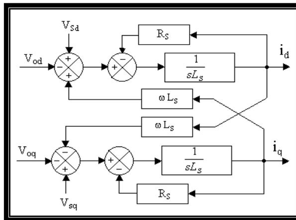
Fig.2: Equivalent Diagram on a.c.side of STATCOM
