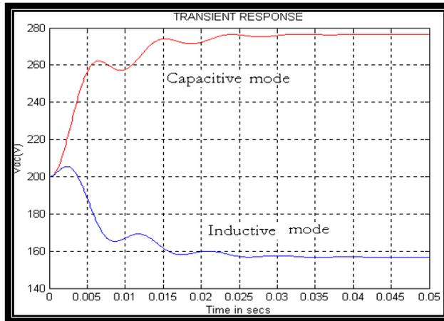
**Fig.10: Transient response of  $v_{dc}$  in both modes**
