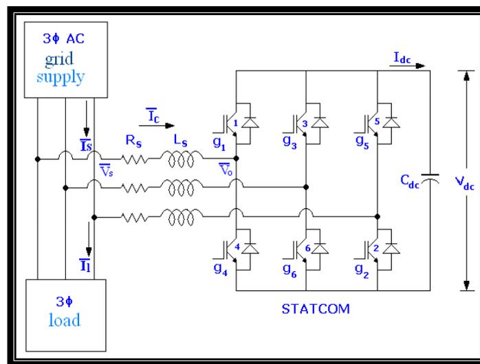
**Fig. 1: Configuration of STATCOM**
