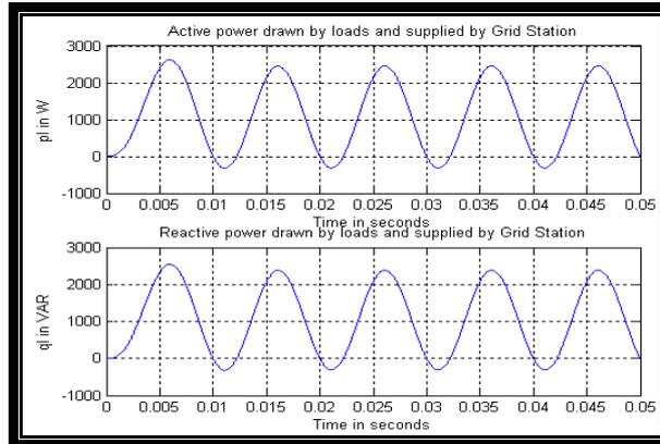
**Fig.14: Grid supplied active and reactive power to  $R-L$  load before operation of the STATCOM**
