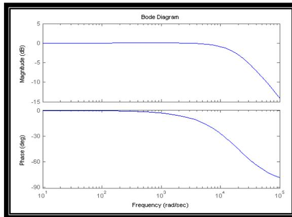
**Fig.6: Bode plot of the system with PI**
