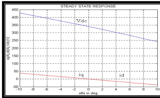
Fig.7: Steady state response of  $i_d$  and  $i_q$
