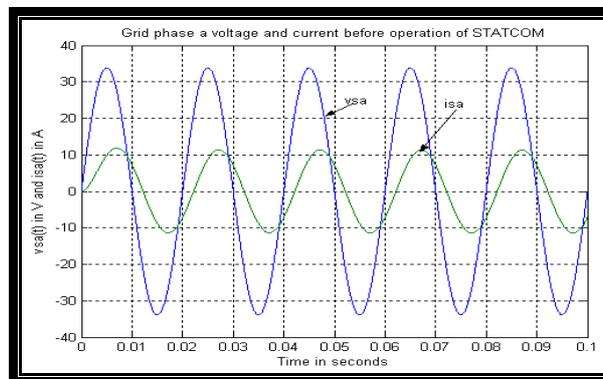
**Fig.13: Grid phase-a voltage and current with  $R-L$  load before operation of the STATCOM**
