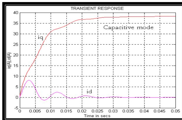
Fig.8: Transient response of  $i_d$  and  $i_q$  in capacitive mode
