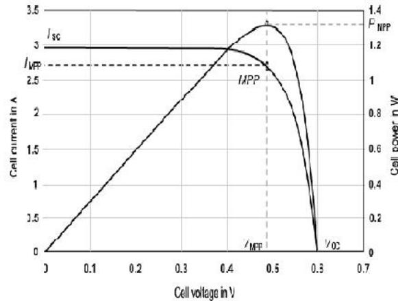
**Fig 2: (I-V) and (P-V) Characteristics of Solar Cell**
