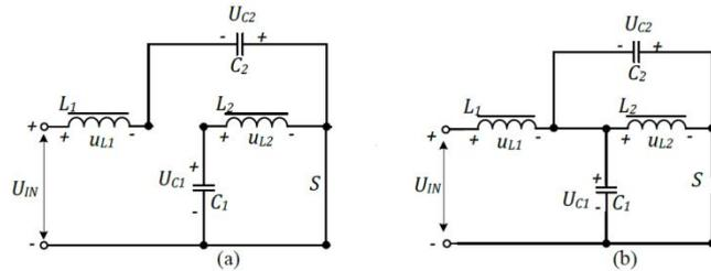
**Fig 5: Quasi Z-source Converter operational stages a) Shoot Through stage b) Non Shoot through stage**
