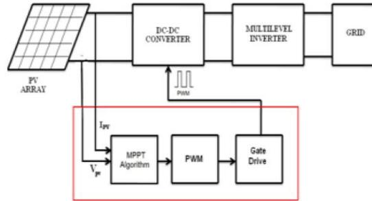
**Fig 1: Proposed PV System for Grid Integration**
