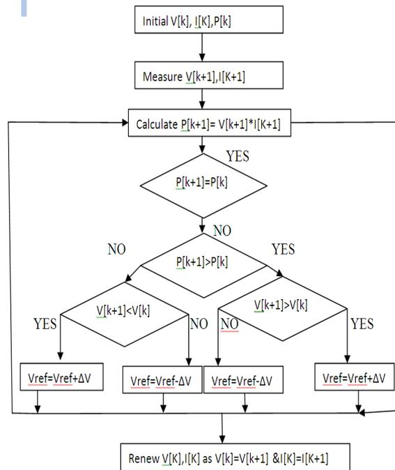
**Fig 3: Algorithm for P&O Method**
