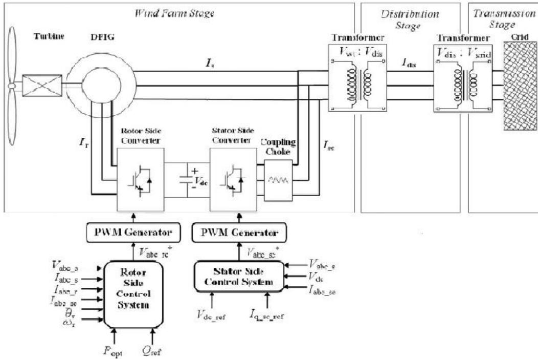
Fig. 2. Wind Turbine Doubly Fed Induction Generator System Configuration
