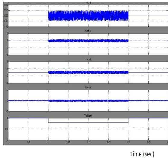
**Fig. 9.** Dynamic response to grid voltage drop (a). dc-link voltage Vdc (b). rotor speed Wr (c). active power P (d.) reactive power Q (e). grid voltage Vgrid
