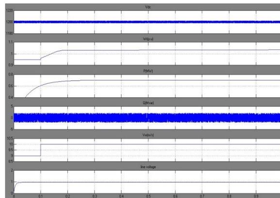
**Fig. 8.** wind step response (a) dc-link voltage  $V_{dc}$  (b) rotor speed  $W_r$  (c) active power  $P$  (d) reactive power  $Q$  (e) wind speed  $V_w$ . (f) distribution line voltage.
