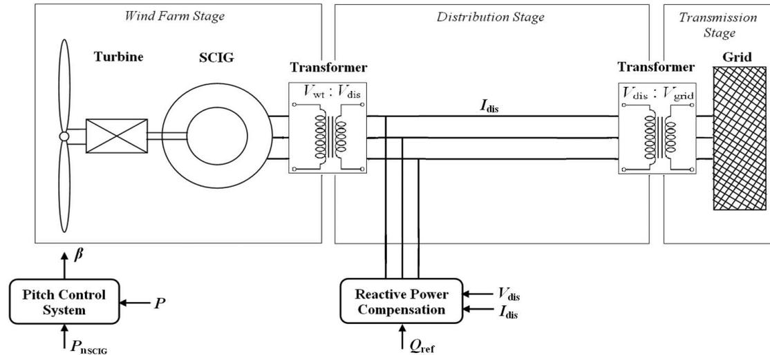
**Fig. 1.** SCIG wind power system model
