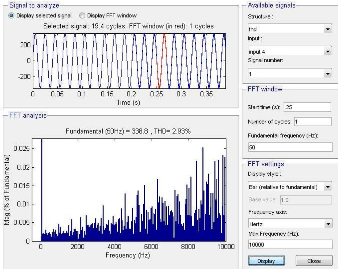
**Fig. 13.** THD improvement for non-linear load
