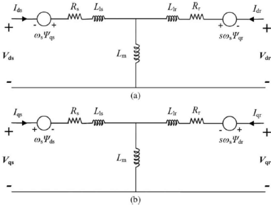
Fig. 3. Equivalent circuit of DFIG a. d-axis and b. q-axis models
