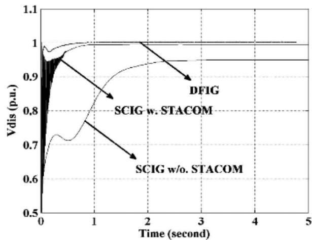
**Fig. 7.** Distribution voltages for SCIG system with and without STATCOM and DFIG
