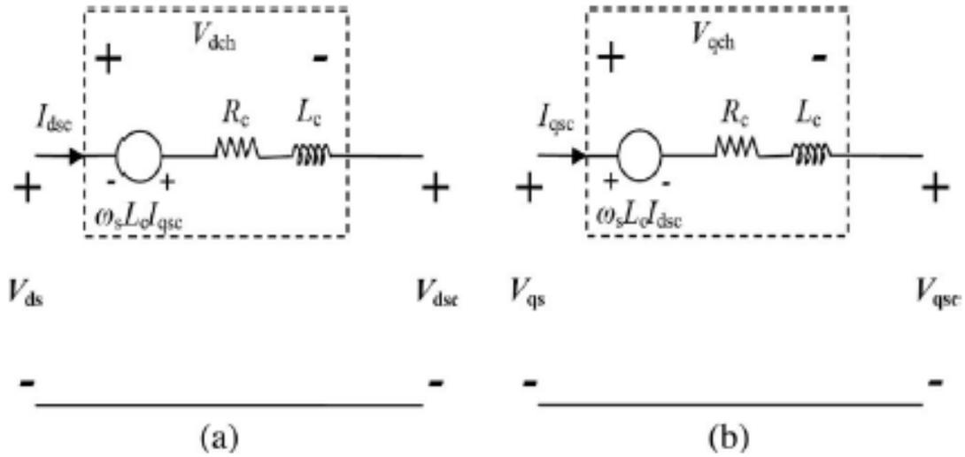
Fig. 5. Stator side Converter Control Scheme (a) d-Axis Model (b) q-Axis Model
