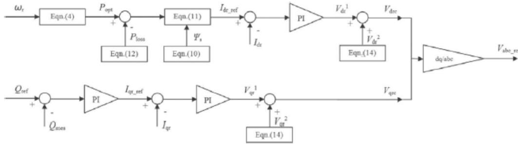
**Fig. 4.** Rotor side converter control scheme
