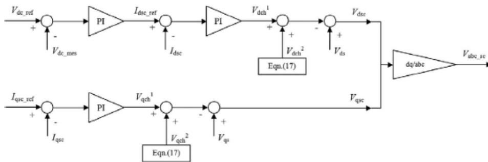
Fig. 6. Stator side converter control model
