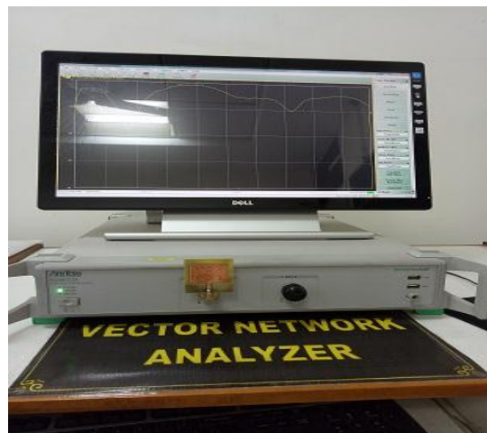
Figure 7. Testing setup for analyzing the return loss and VSWR of proposed antenna
