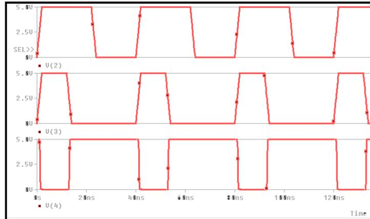
**Figure 12:** Behavior of CNTFET based NOR gate.
