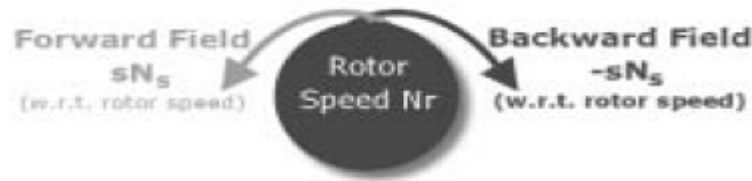
Fig 7. shows the Illustration of forward and backward rotating magnetic fields from rotor currents when a Broken Bar exists.
