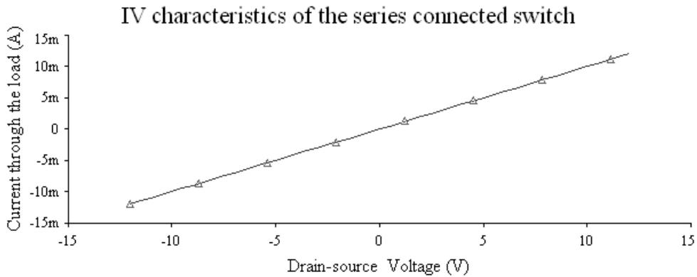
**Figure 3:** DC characteristics of mosfet
