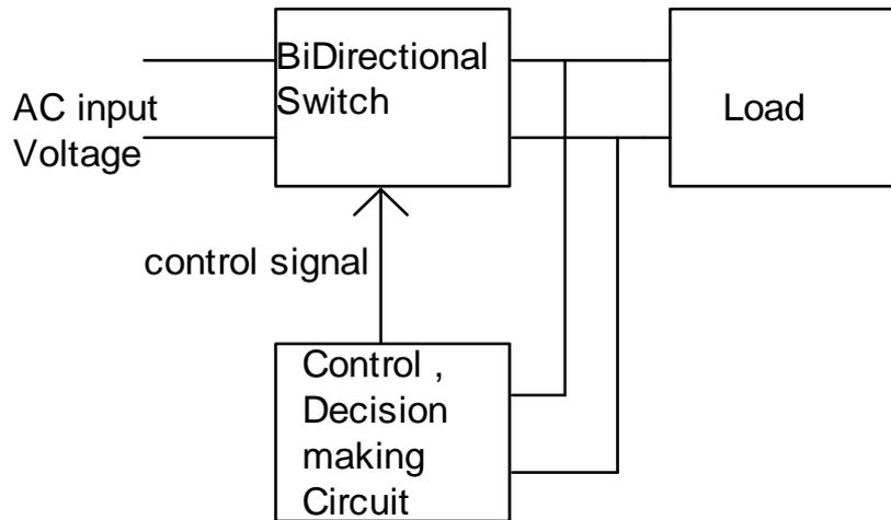
**Figure 1:** Block diagram of the circuit breaker
