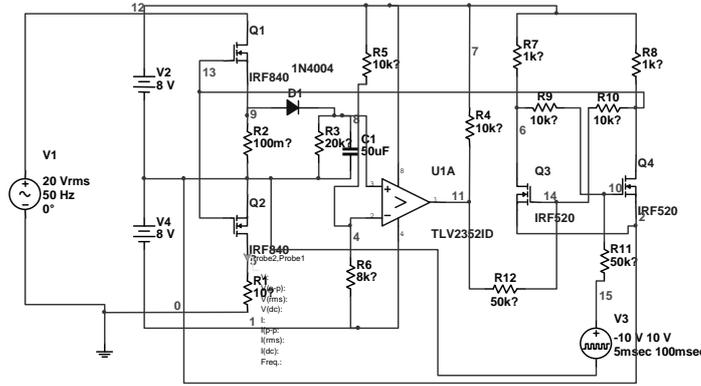
**Figure 2 :** circuit breaker with two mosfets
