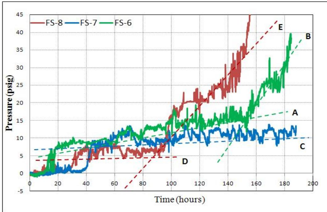
**Fig.3**Effect of flow rate and flux time on scale deposition in copper tube
