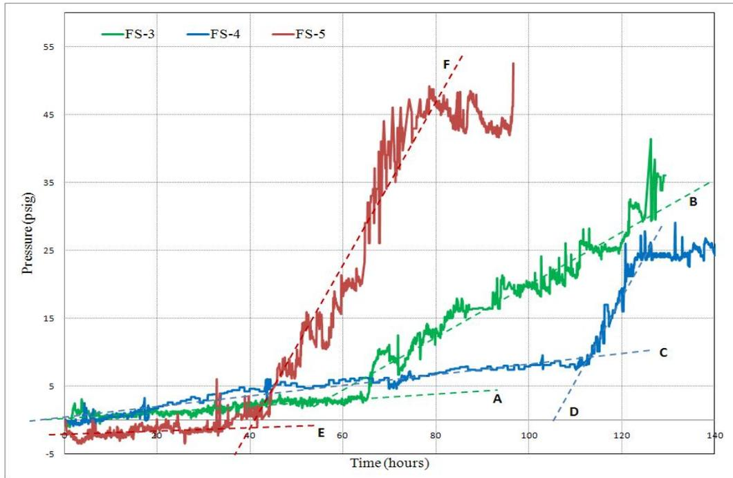
**Fig.2.**Effect of flow rate and flux time on scale deposition in plastic tube.
