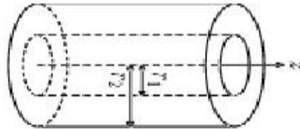
Each layer of the fluid has its own radius and velocity. Eq. 3 can be re-written for each layer as:
