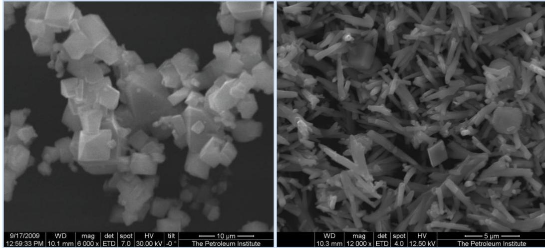
**Fig.4.** SEM images of scale crystals under (A) no magnetic field (calcite) and (B) under magnetic field (predominantly aragonite).
