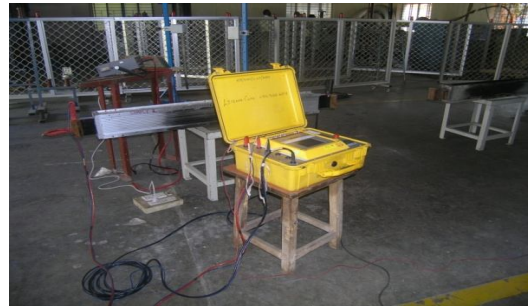
Fig. 4: Test setup for - Conductor resistance measurement
