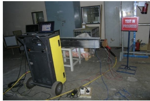
Fig. 3: Test setup of Capacitance & \tan\delta measurement
