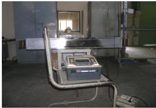
Fig. 2: Test setup of IR & PI measurement
