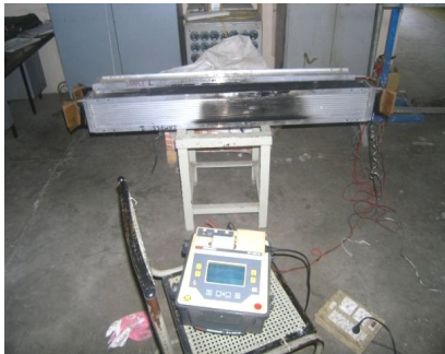
Fig. 1: Test setup of IR & PI measurement
