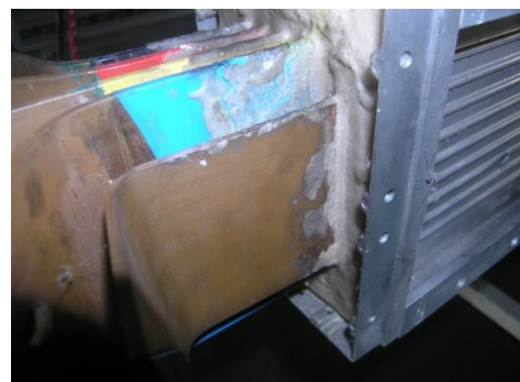
Fig. 8: The terminal ends of busduct model with dielectric envelop after fire survival test
