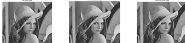
Fig. 5: The decoded “LENA” from left to right (a) original (b) modified OFDM [PSNR= 30.4160 dB] (c) Modified OFDM with adaptive clipping [PSNR= 29.9306 dB] over AWGN channel at SNR=15 dB with QAM16
