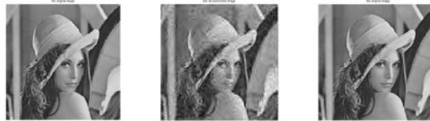
Fig. 3: The decoded “LENA” from left to right, (a) original, (b) Original OFDM [PSNR= 24.5140 dB], (c) Modified OFDM (UEP) [PSNR= 30.4160 dB]
