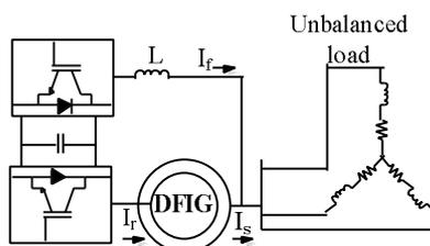
**Fig. 1:** DFIG sourcing a stand-alone unbalanced load.
