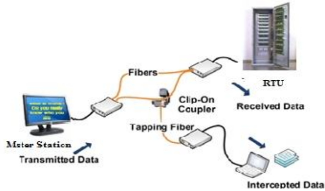
Fig. 3: Fiber optic tapping.
