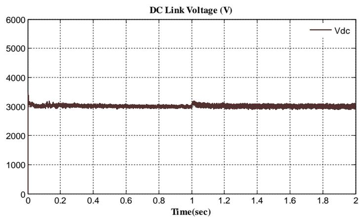
Fig. 6. 3 DC Link voltage
