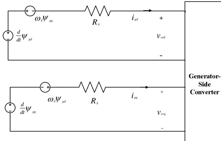
**Fig. 3.** Equivalent circuit of PMSG in synchronous frame
