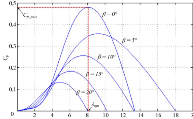
**Fig. 2.** Power coefficients over tip speed ratio at various pitch angles
