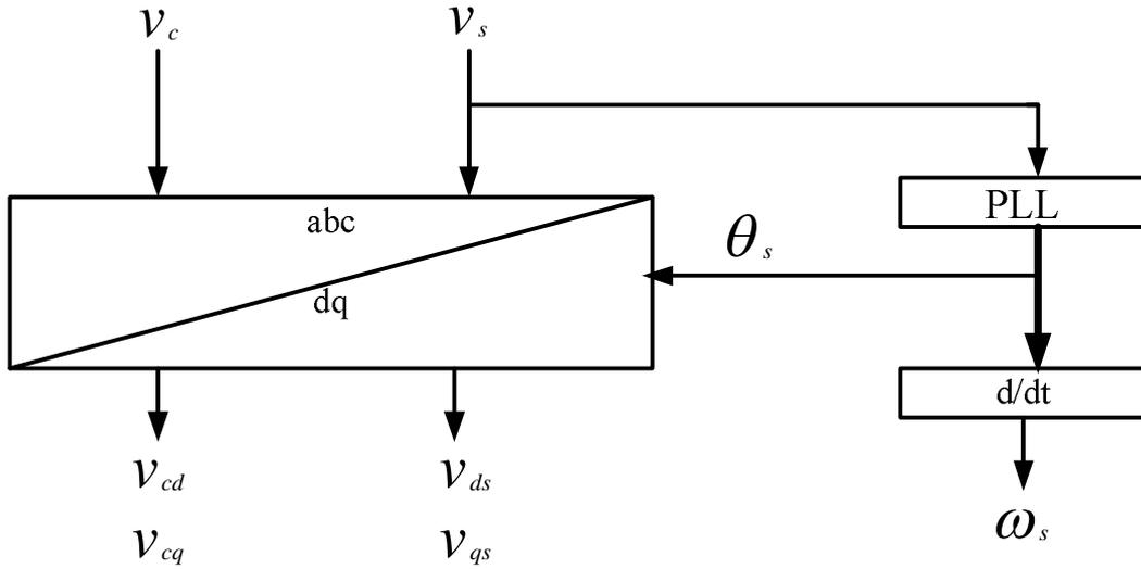
**Fig.. 7.** Grid voltage PLL and coordinate transformation
