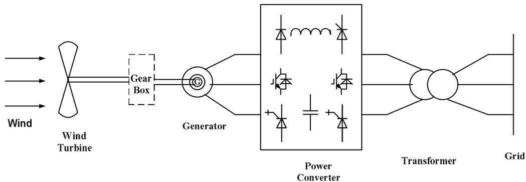
**Fig. 1.** Basic configuration of the contemporary WECS
