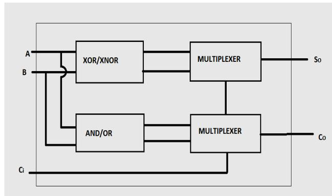
**Figure 2:** Alternative logic structure for designing full-adder cell
