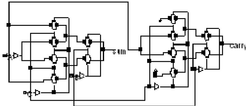
**Figure 4:** Full-adder designed with the proposed logic structure
