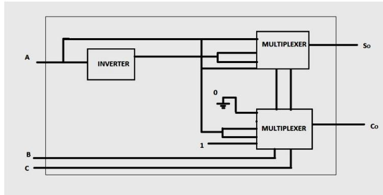
**Figure 3:** Logic structure for proposed full-adder cell
