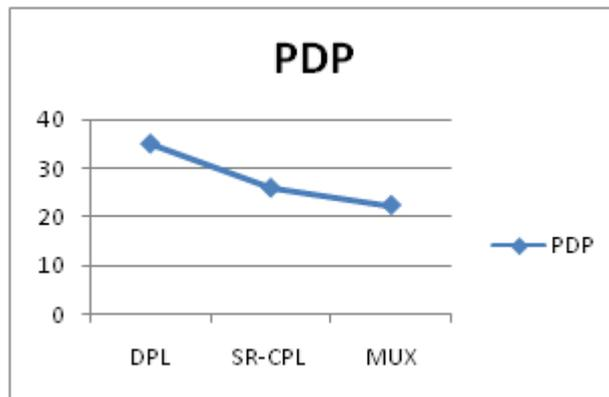
Figure 5: Power-delay product(PDP) comparison
