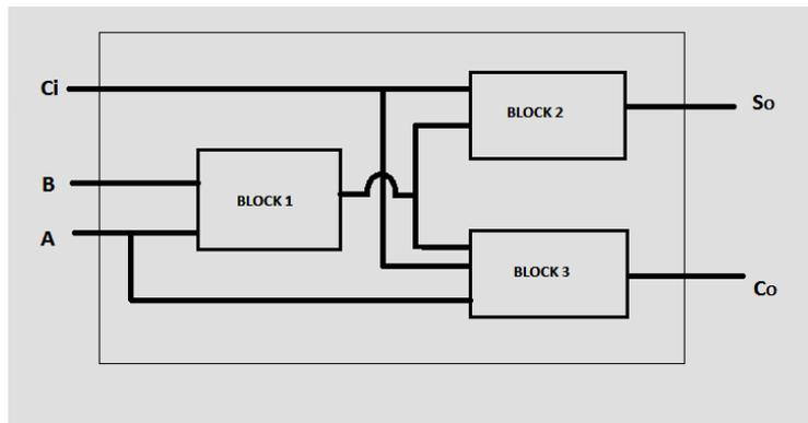
Figure 1: Full-adder cell formed by three main logical blocks
