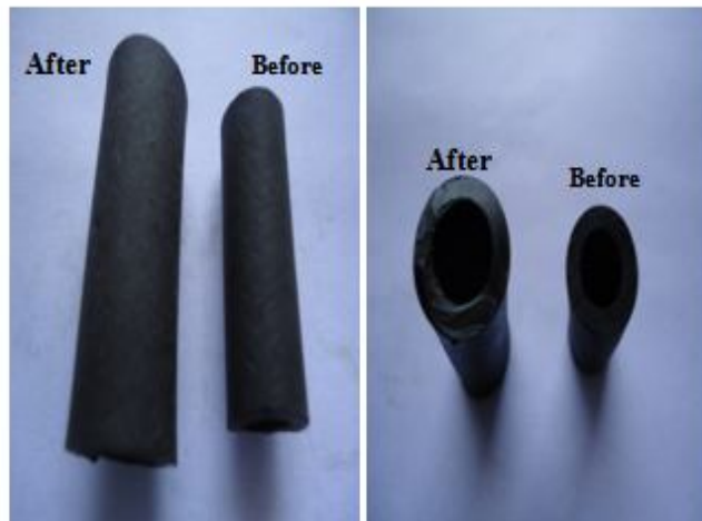
Fig-3: Immersion Test Results for fuel pipe Sample with JOME+E20
