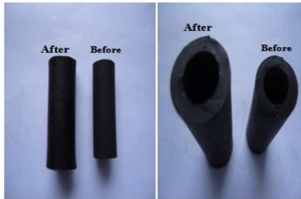
Fig-1: Immersion Test Results for fuel pipe Sample with plain Diesel.
