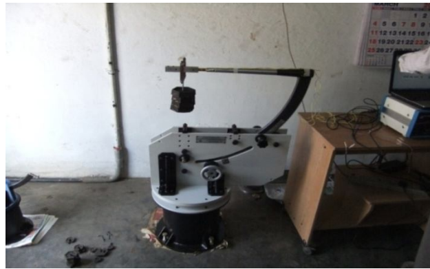
Figure 4: Model Positioning System under Load Test.
