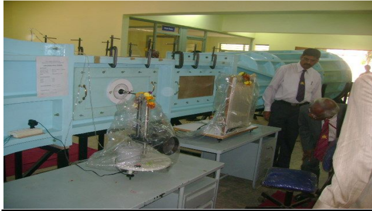
Figure 2: Wind Tunnel at MVJ College of Engineering 6m x .6m x 2m Test Cross-section 50 m/sec Max Speed.
