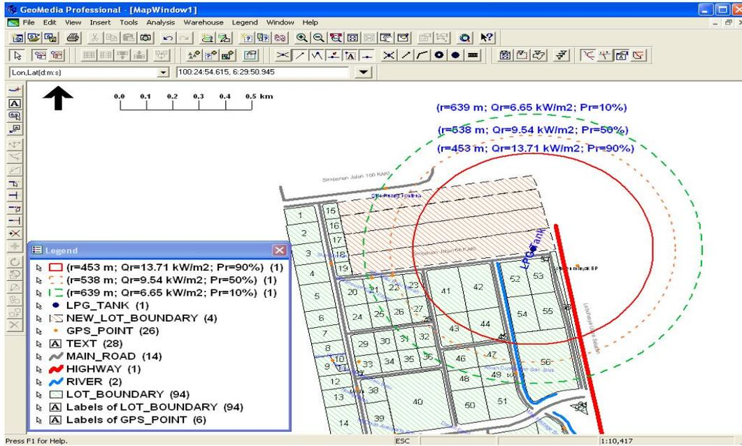
Figure 3: Buffer zones for probability of human protected by clothes from thermal radiation around LPG tank.
