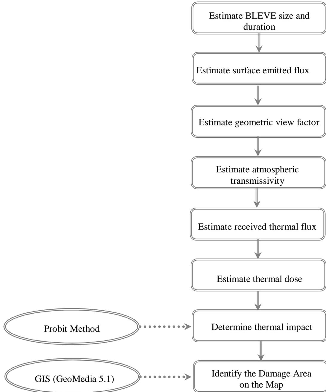
**Figure 1:** Logic diagram for the calculation BLEVE/fireball thermal intensity and thermal impact.
