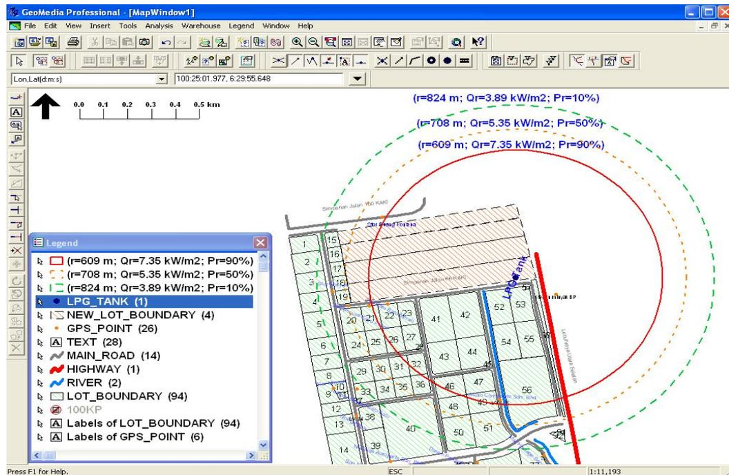
Figure 8: Buffer zones for probability of 1<sup>st</sup> degree of burn.
