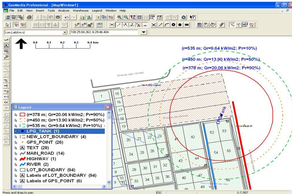
Figure 4: Buffer zones for probability of human unprotected by clothes from thermal radiation around LPG tank.
