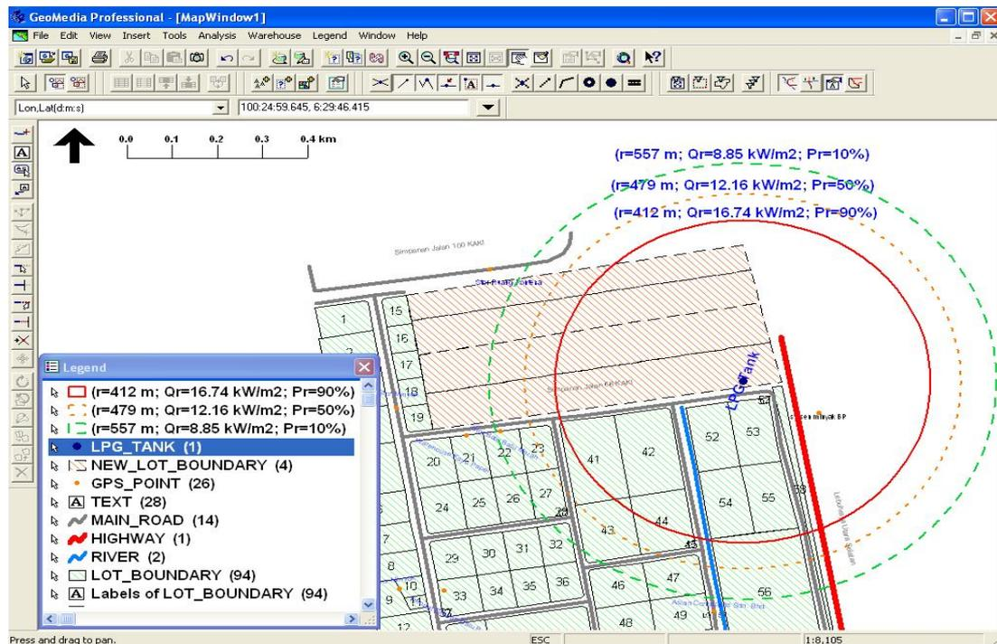
Figure 5: Buffer zones for probability of 2<sup>nd</sup> degree of burn.
