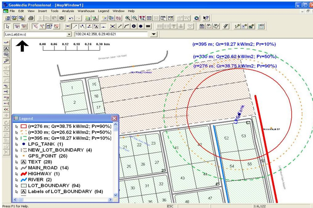
**Figure 6:** Buffer zones for probability of human fatality from thermal radiation around LPG tank.
