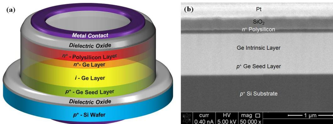
**Fig. 4. (a) Schematic representation of final SiGe PIN photodetector device (not drawn to scale); (b) focused ion beam (FIB) cross-sectional image of fabricated SiGe photodetector device covered with a layer of platinum.**
