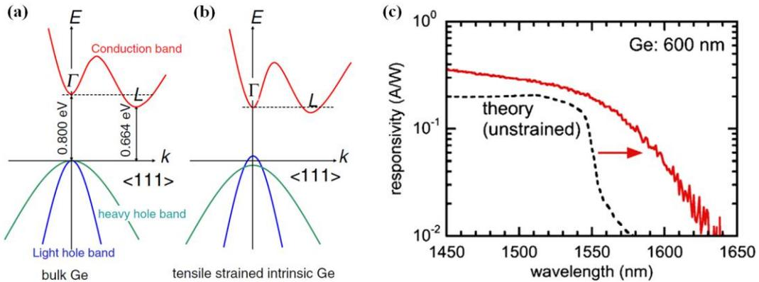
**Fig. 2.** (a) Schematic band structure of bulk Ge, showing 136 meV difference between direct and indirect band gaps; (b) shift of Ge from indirect gap toward direct gap material with application of tensile strain.<sup>18</sup> (c) Comparison of responsivity spectra for PIN photodetectors having unstrained and strained Ge layers.<sup>19</sup>
