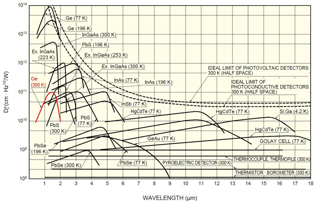
**Fig. 1. Detectivity curves for various commercially available IR detectors plotted vs. wavelength. Calculated ideal detectivity limits are indicated by dashed lines.<sup>4</sup>**
