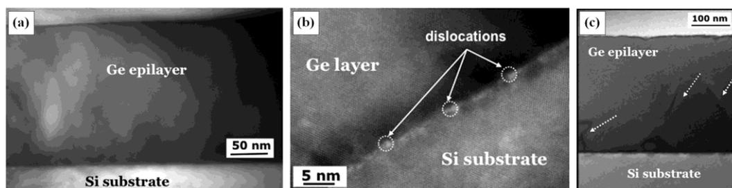
**Fig. 3.** (a) Cross-sectional transmission electron microscopy (TEM) image of Ge layer grown on Si; (b) enlargement of layer in (a) near the interface region, showing a high density of misfit dislocations; and (c) TEM image of the Ge layer grown following a two-step growth process, where threading dislocations are less evident.<sup>17</sup>
