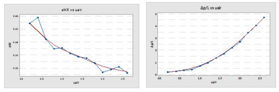
Fig. 3 Effectiveness versus velocity Fig. 4 Pressure drop per unit length versus velocity
