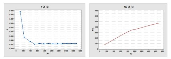
Fig. 5 Friction factor versus Reynolds number Fig.6 Nusselt number versus Reynolds number
