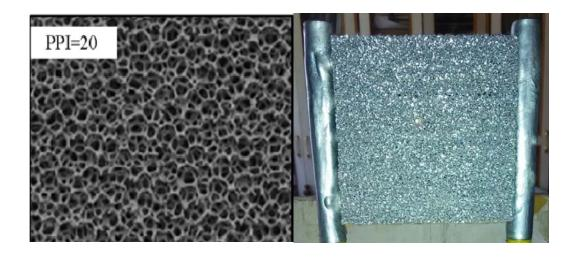
Fig. 1Sructure of an 20 PPI metal foam and a heat exchanger fabricated out of it.
