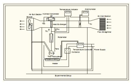
Fig. 2. Experimental Setup used in the study.[12]
