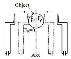
Fig. 2 Reaction forces on grasping process of parallel gripper.
