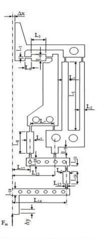
Fig. 5. The design variables of the compliant parallel micro-gripper mechanism.
