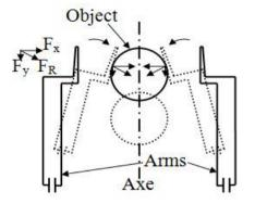
Fig. 1 Reaction forces on gripping process of unparallel gripper.
