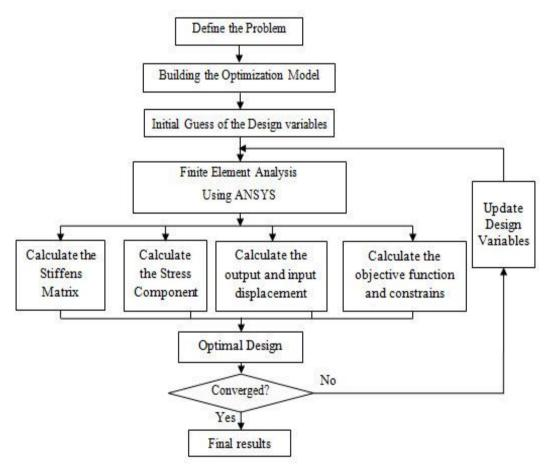
Fig. 9. The design optimization flow chart for the compliant micro-gripper mechanism.
