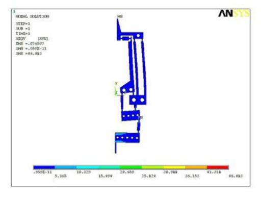
Fig. 12 Von-Mises stress distribution of compliant micro-gripper mechanism.
