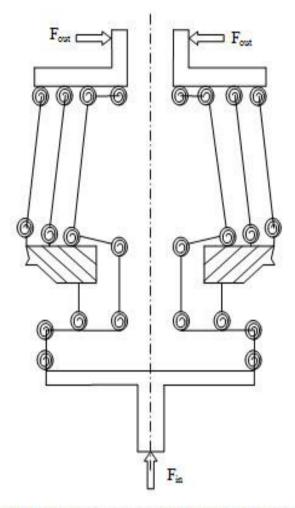
Fig. 7 Kinematic representation of the micro-gripper compliant mechanism.
