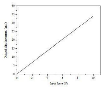
Fig. 13. The output displacement versus the input force for the micro-gripper mechanism.
