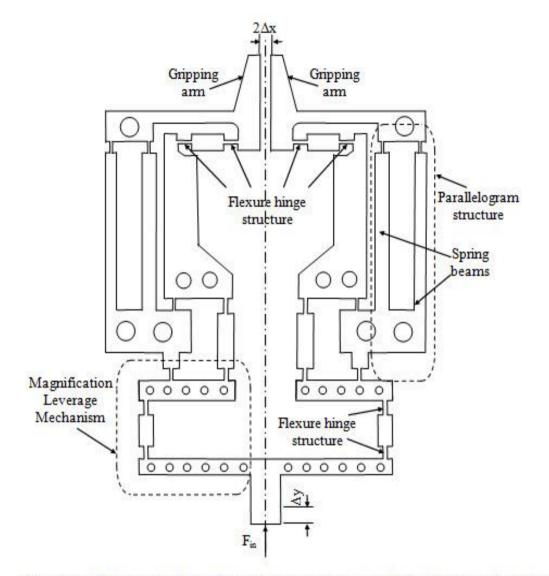
Fig. 4 The full geometrical configuration model of the compliant parallel micro-gripper mechanism.
