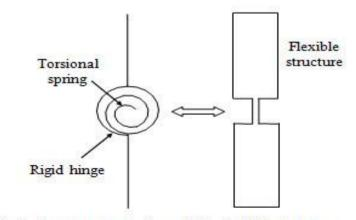
Fig. 6 Equivalent representation of the flexible structure.
