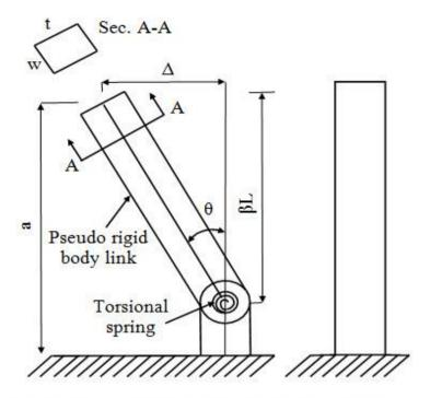
Fig. 8 Pseudo rigid body model (PRBM) of the spring beam structure.
