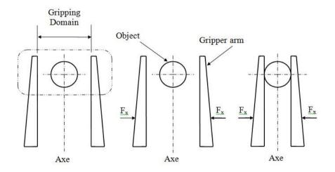
Fig. 3. The grasping of micro-object process: (a) The micro-gripper will be positioned within the grasping domain, (b) both jaws approaching the object for providing the necessary contact without damage, and (c) finally, both jaws perform sub-micrometer motion to firmly hold the object into position without slippage and damage.
