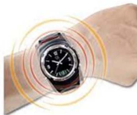
Figure 38. Vibrating watch for pedestrian warning
