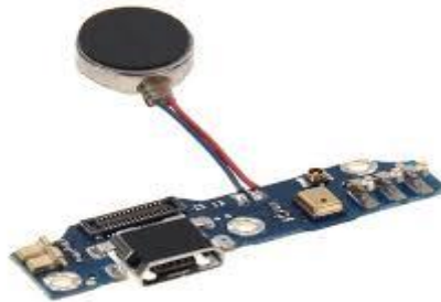
Figure 39. Vibration device for pedestrian warning
