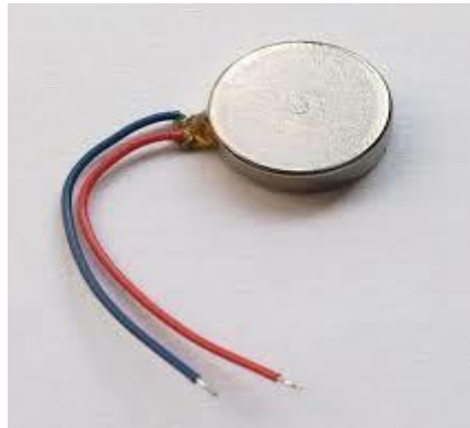
Figure 36. Vibration device for pedestrian warning
